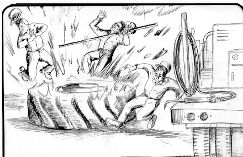
Heating of wheel fastening systems is a key root cause to many tyre and rim related fatalities. This work practise must be eliminated. Sketch from [3].
