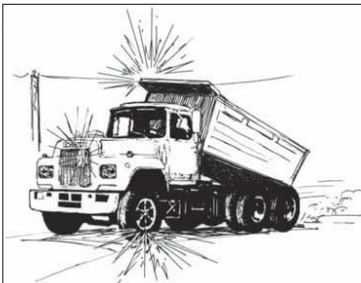
Accidental contact with overhead powerlines or electrification by lightning strike is known to cause pyrolysis and subsequent violent explosion of in some or all vehicle tyres. This hazard can be best eliminated by designing roads away from powerlines. (sketch from [2])
