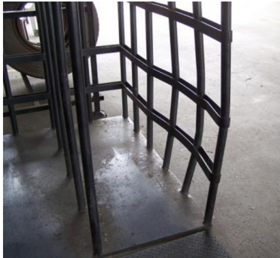
Example of engineer-certified tyre inflation cage after testing with a 22.5 inch tyre at 140 PSI. Image courtesy RLM Distributing.
