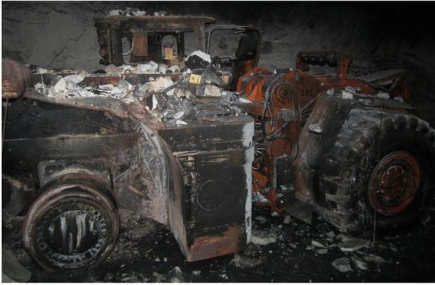
**Fig. 18** The right-hand side of the loader with the front mudguard partially affected by the fire. Photo: Andreas Fransson [26]
