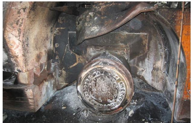
**Fig. 11** The left, rear wheelhouse of the loader after the full-scale fire experiment. Photo: Andreas Fransson
