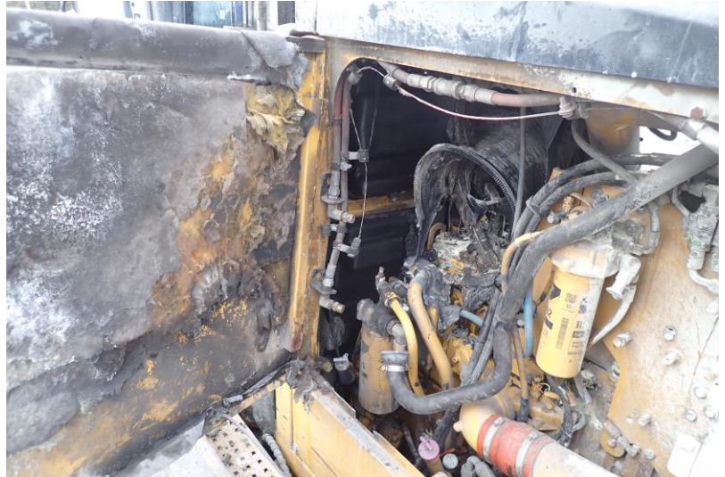
Figure 2: Grader fire damage and location
