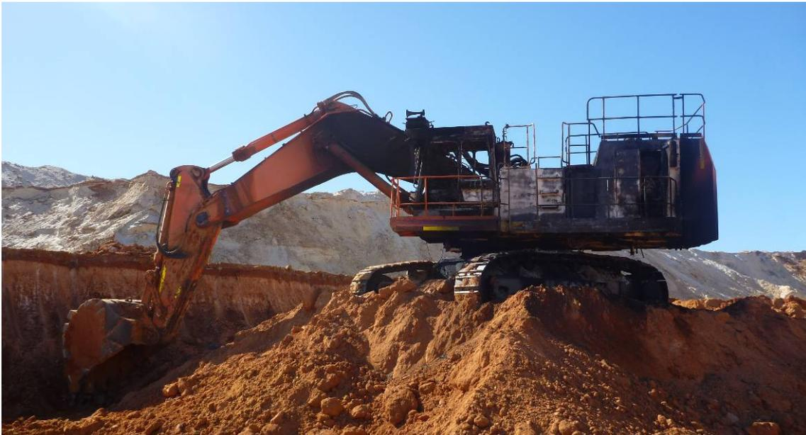
*Photo 1 - Excavator after fire was extinguished.*
