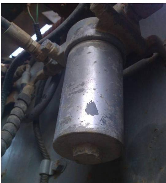
Photo 2 – Oil filter housing cast removal nut.
