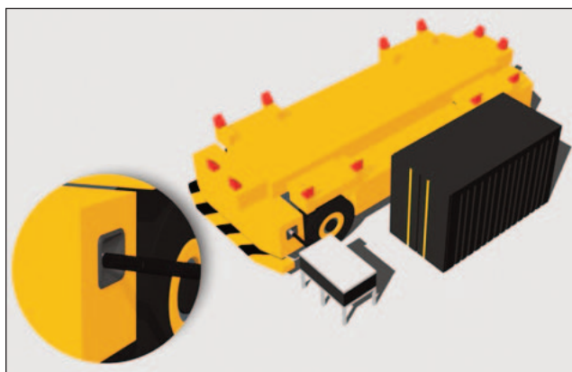
Figure 22. Automated Enclosed Pin and Socket Charging Interface
