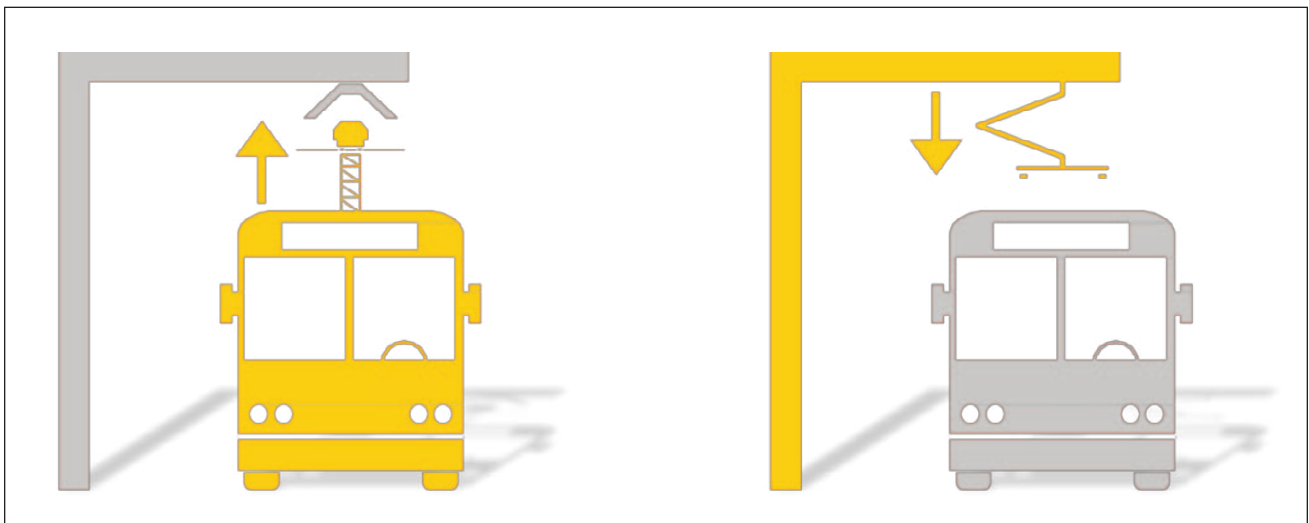
Figure 19. Two Pantograph Interfaces Available and Standardized in SAE J3105 (Table 8)
