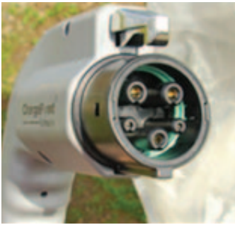
Figure 15. SAE J1772 Connector (SAE International, 2017)
