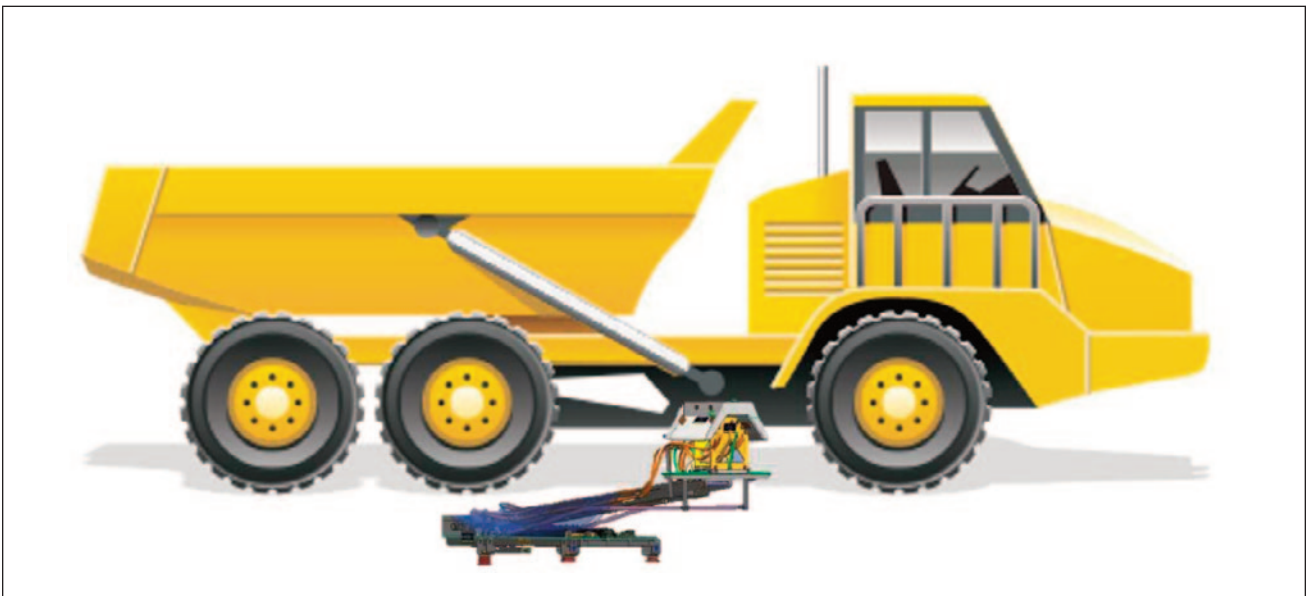
Figure 21. Underbody Charging Using a Bottom-Up Pantograph
