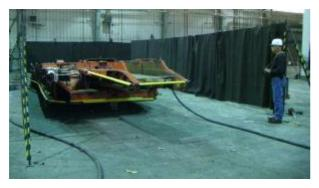
Researchers evaluate the Intelligent Proximity Detection system installed on a continuous mining machine in a simulated mine environment.
