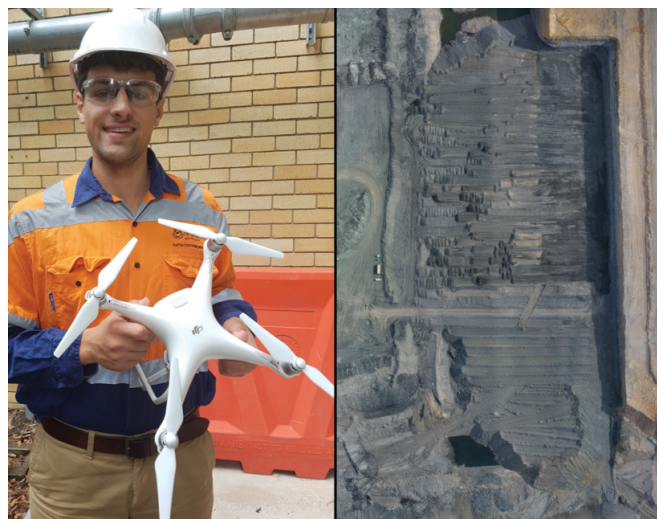
FIG 2 – An example of the capabilities of current unmanned aerial vehicle systems. This particular system, easily carried by hand (see left), is used to develop high accuracy digital terrain maps and high quality visual imagery (see right). This particular mission, at a coalmine in Australia, was to provide daily volumetric reconciliations of waste material moved. The mission could be completed in 30 minutes, with minimal survey support required for installation and maintenance of reference targets on the ground.
